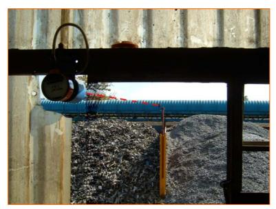
the switch. The MicroSense's switching capabilities are unaffected by dust, steam, smoke or heat, whilst build up of material on the antennae has little or no effect on the operation.
