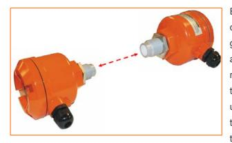
Each switch subsystem is comprised of two components, a microwave transmitter, which generates a low power 24 GHz microwave beam, and a receiver unit with a maximum operating range of 40 metres between the two antennae. The two units are mounted facing each other and in the un-switched state the narrow beam from the transmitter is detected by the receiver. If the path of the beam is then interrupted by a sufficiently
